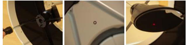
**STEP 9: Removal of the laser collimator from focuser**
